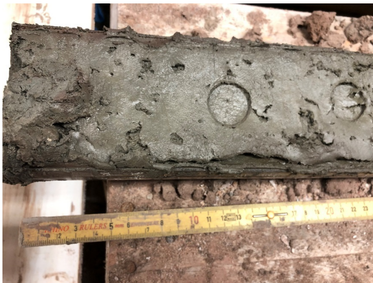
Photo 3 Representative core sample from location VC-20A-3, illustrating top 0.2 m portion of the 1.5 m to 3.5 m section of core containing soft, grey, clayey silt
