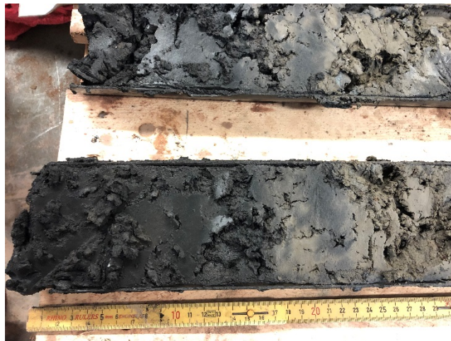
Photo 5 Representative Core Sample from Location VC-50C-3, illustrating the top 0.3 m of bottom depth core (1.2 to 2.2 m) containing grey to black silt
